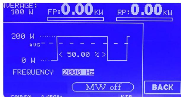
Set up of the pulse on the digital display
